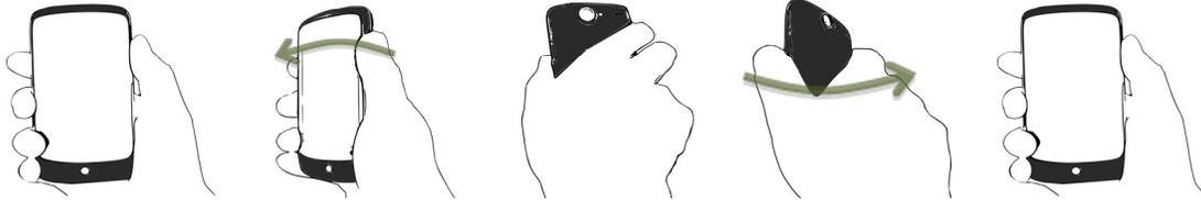
Figure 1: An illustration of the DoubleFlip gesture. In this figure, the user holds the phone right-handed. He rotates the phone along its long side so that the phone screen is away and then back.
